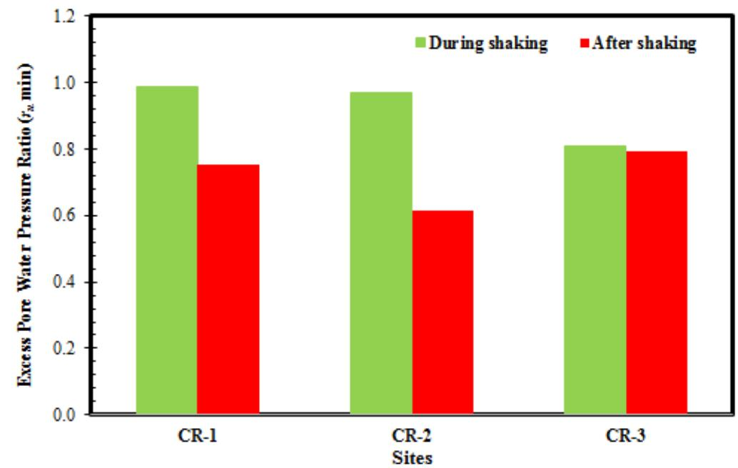
Minimum excess pore water pressure ratio during and after shaking
