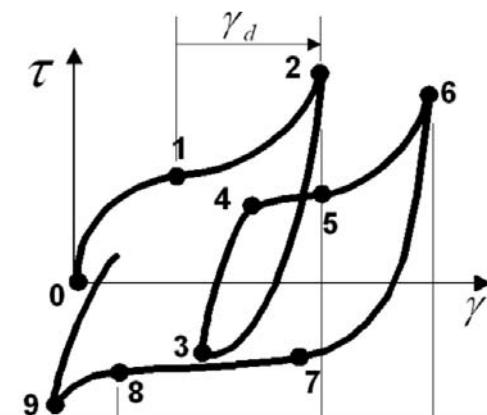
Stress-strain curve of shear strain model for sand under cyclic mobility (Elgamal et al., 2006)
