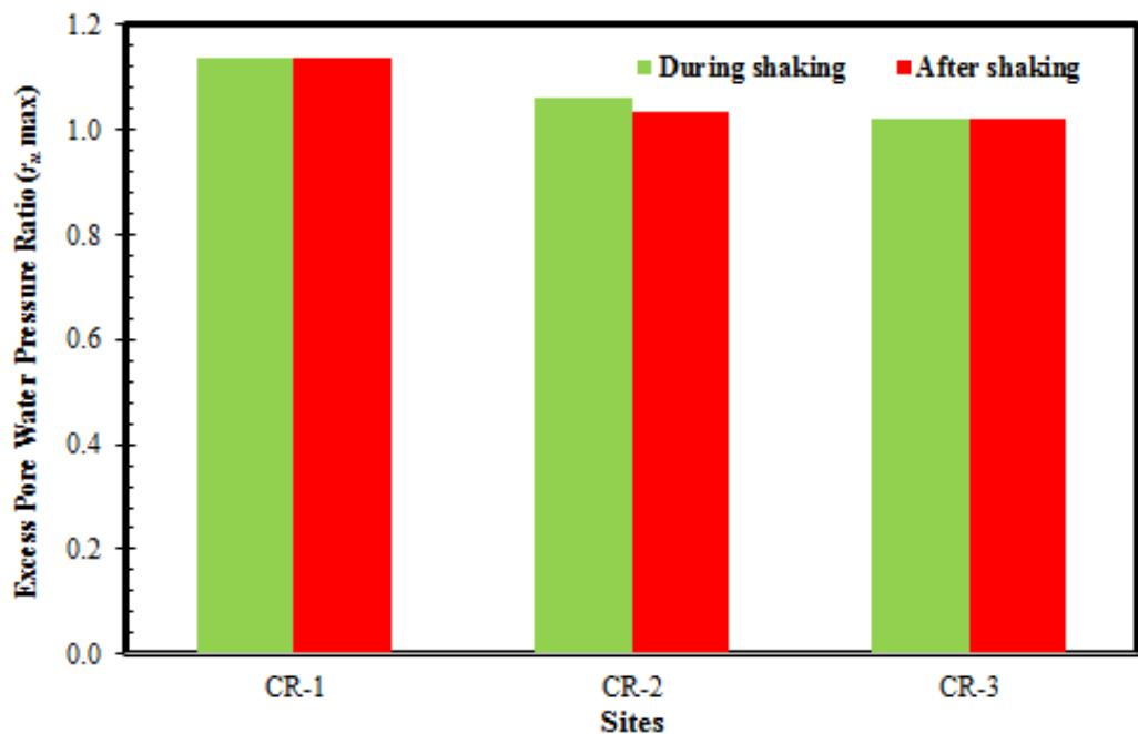
Maximum excess pore water pressure ratio during and after shaking
