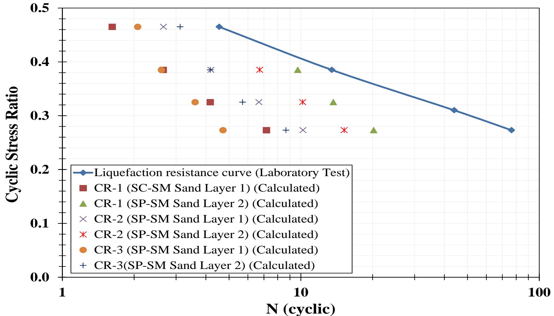
Fig.7 Liquefaction resistance curve comparison for all liquefiable layers from element simulations
