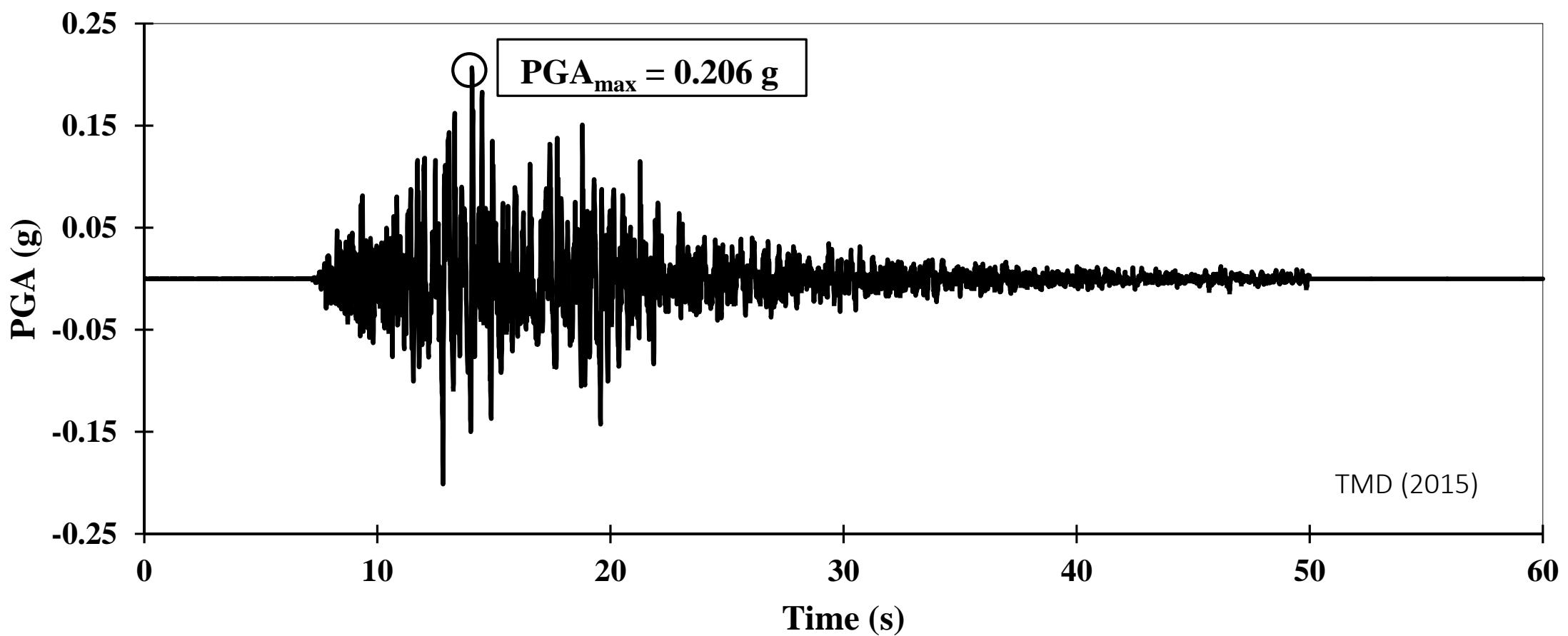
Fig.3 Acceleration record of Mae Sai Station during the  $6.8 \text{ M}_w$  earthquake on 24 March 2011<sup>6)</sup>.
