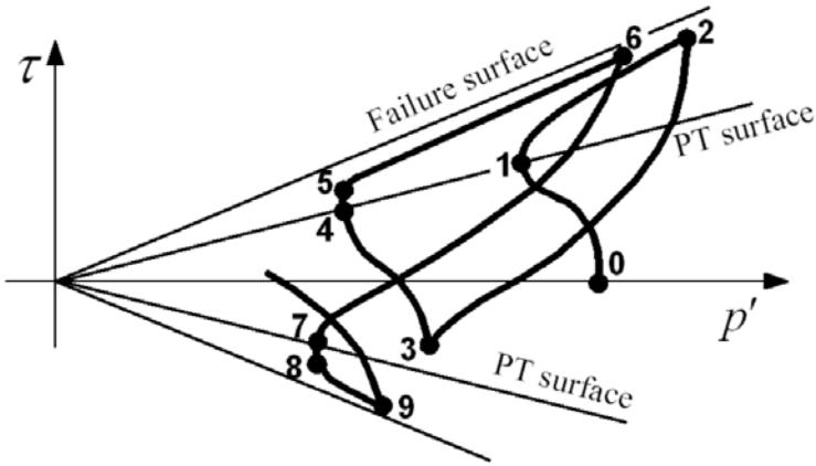
Effective stress path of shear strain model for sand under cyclic mobility (Elgamal et al., 2006)
