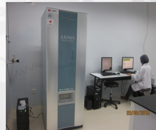
Matrix Assisted Laser Desorption/Ionizing Time Of Flight – Mass Spectrometry (MALDI TOF – MS)
