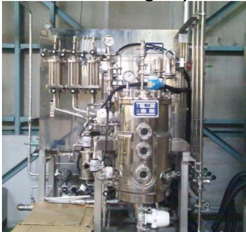
50 L fermentation reactor
